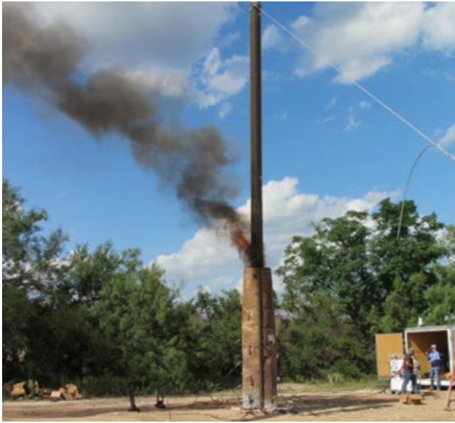
Fire Resistant Pole System being tested.
