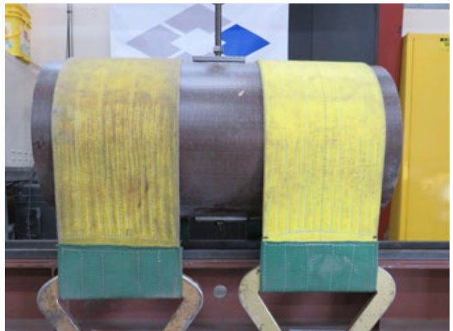
Bolt Pull Through Testing at EDM International
